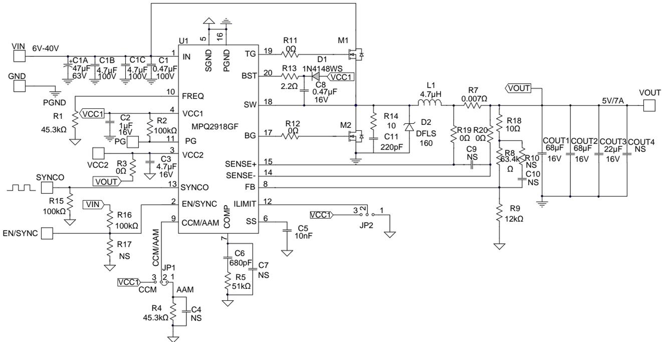
Note: Thermal pad should connect to PGND and SGND
