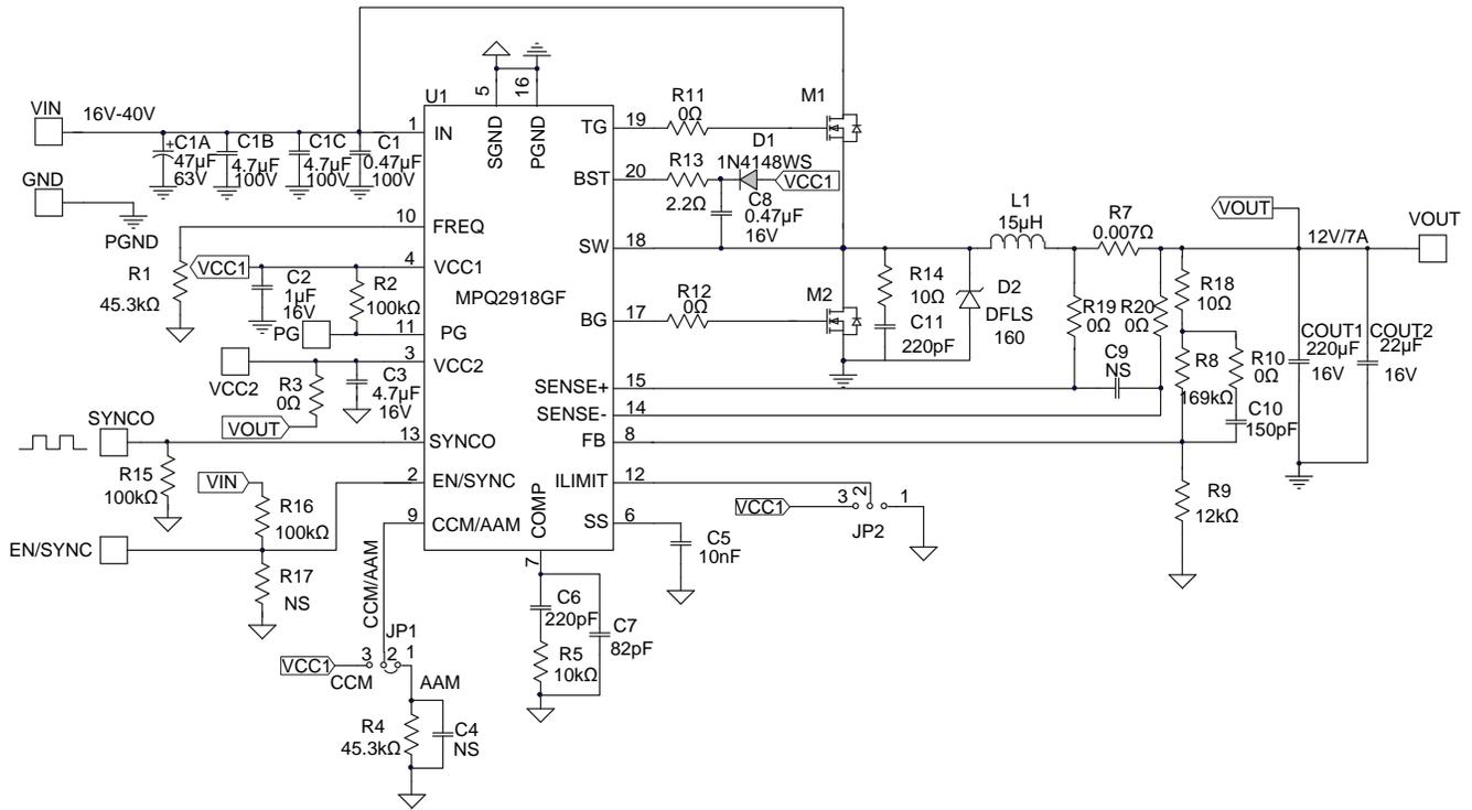
Note: Thermal pad should connect to PGND and SGND
