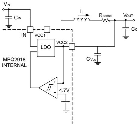
Figure 7: Configuration of VCC2 Connecting to  $V_{OUT}$
