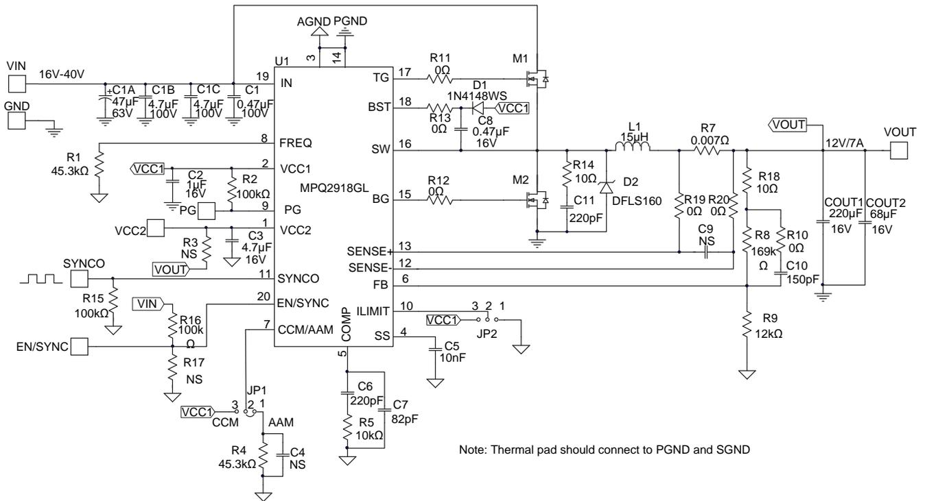
Figure 16: 12V Output Application Circuit for QFN Package
