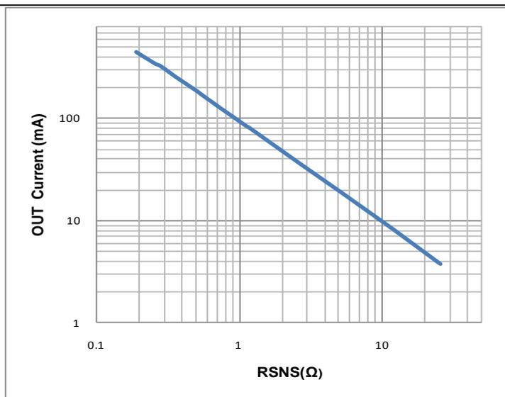
Fig 3. Output Current vs Current-Sense Resistor
