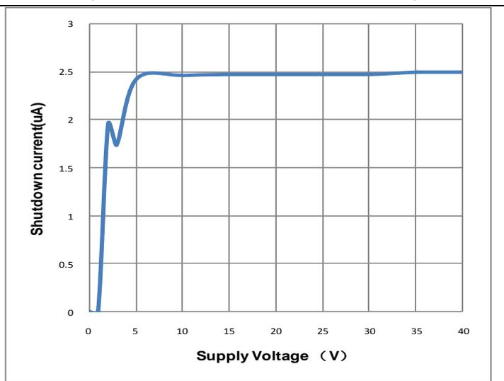
Fig 7. Shutdown Current vs Supply Voltage
