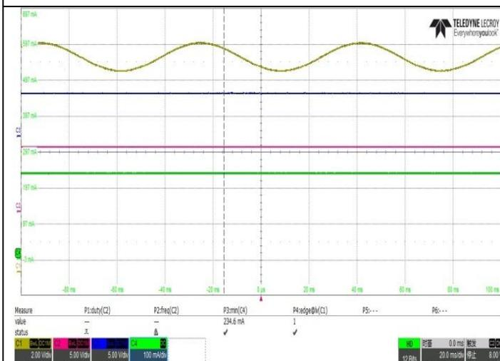
C1-SUPPLY C2-VOUT C3-FAULT C4-IOUT
