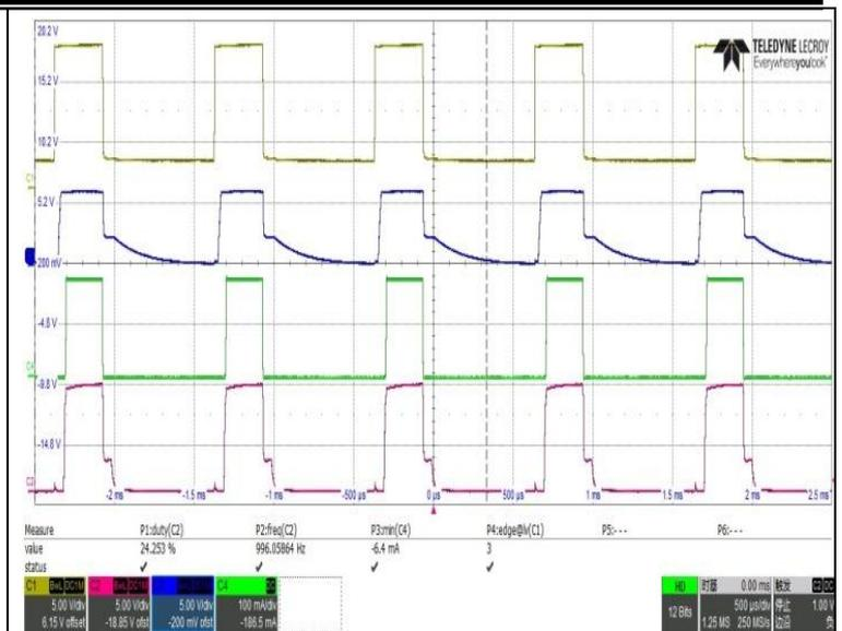
C1-SUPPLY C2-VOUT C3-FAULT C4-IOUT
