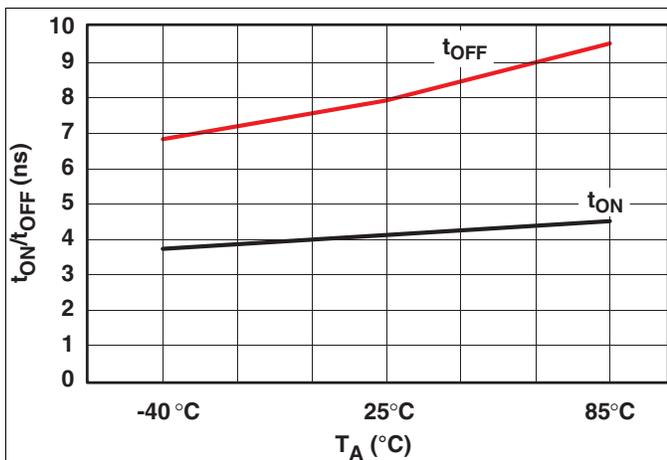
Figure 7. t<sub>ON</sub> and t<sub>OFF</sub> vs Temperature (V<sub>+</sub> = 5 V)
