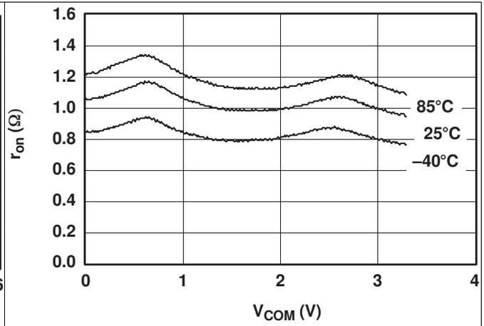
Figure 2.  $r_{on}$  vs  $V_{COM}$  ( $V_+ = 3.3$  V)
