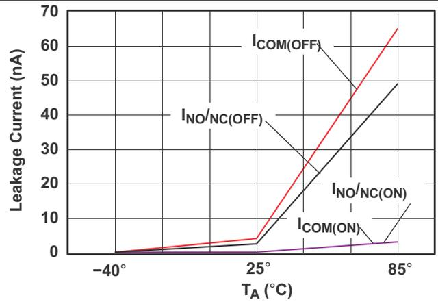
Figure 4. Leakage Current vs Temperature ( $V_+ = 5.5$  V)
