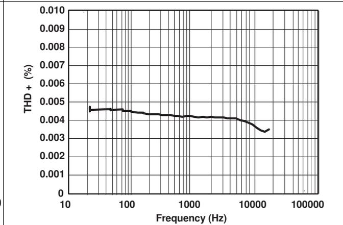
Figure 10. Total Harmonic Distortion vs Frequency
