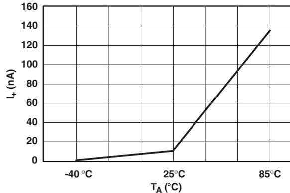
Figure 22. Power-Supply Current vs Temperature (V+ = 5 V)
