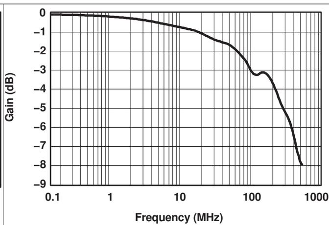
Figure 8. Bandwidth (V<sub>+</sub> = 5 V)
