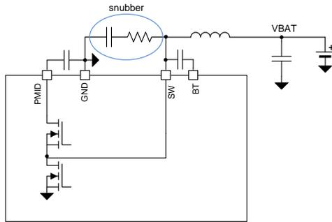
Figure 6. Snubber circuit
