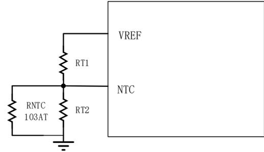
Figure 5. NTC Circuit
