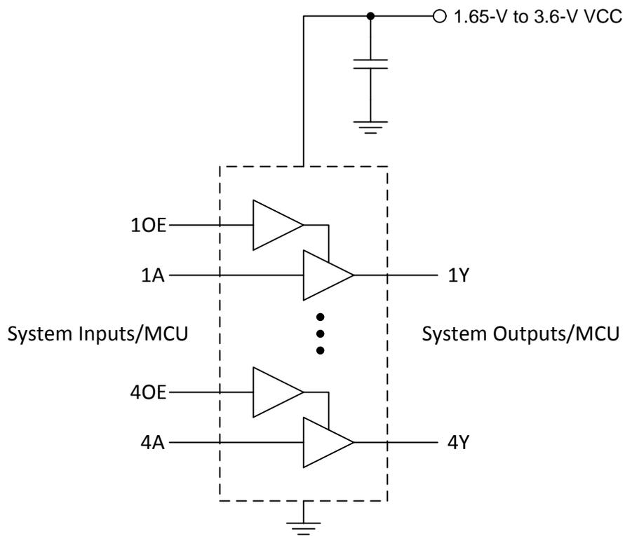
**Figure 7. Typical Buffer Application and Supply Voltage**
