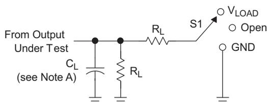
Figure 2. Load Circuit
