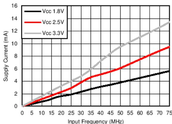
Figure 8. Supply Current vs Input Frequency
