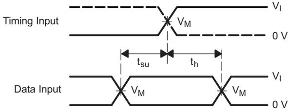
Figure 4. Voltage Waveforms, Setup and Hold Times
