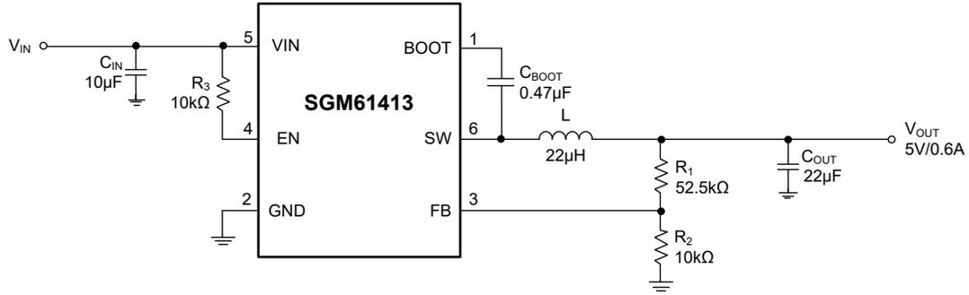
**Figure 4. 5V Output Typical Application Circuit**
