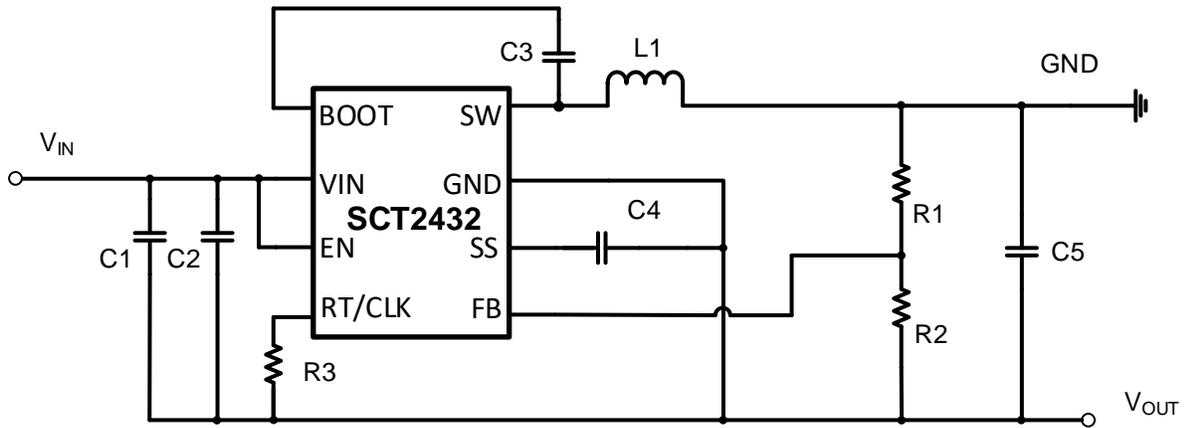
Figure 20. SCT2432 Inverting Power Supply
