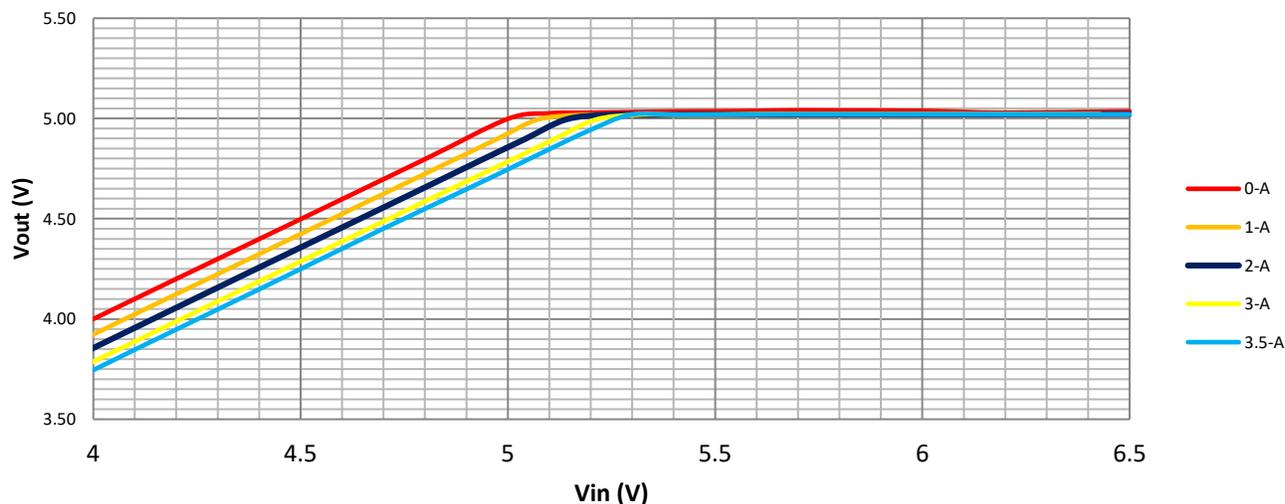
Figure 18. LDO Operation Characteristic ( Vout =5V )
