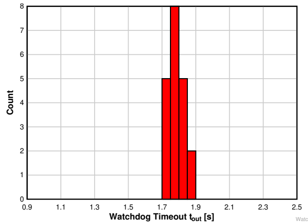
Figure 7-14. Watchdog Timeout Histogram for TPS3823A-33 Devices at 125°C (Unit Count = 20)
