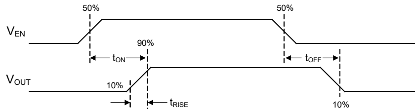
Figure 3. SGM2588A/C/E/G/I/K Switch Turn-On and Turn-Off Delay Times
