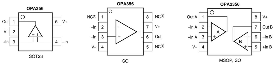
NOTE: (1) NC means no internal connection.
