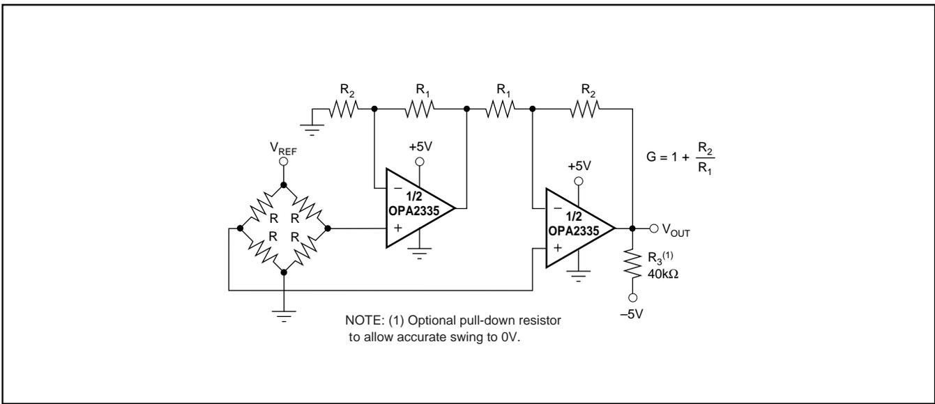
FIGURE 6. Dual Op Amp IA Bridge Amplifier.
