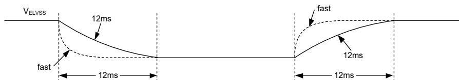
Figure 3. V_{ELVSS} Transition Time Control
