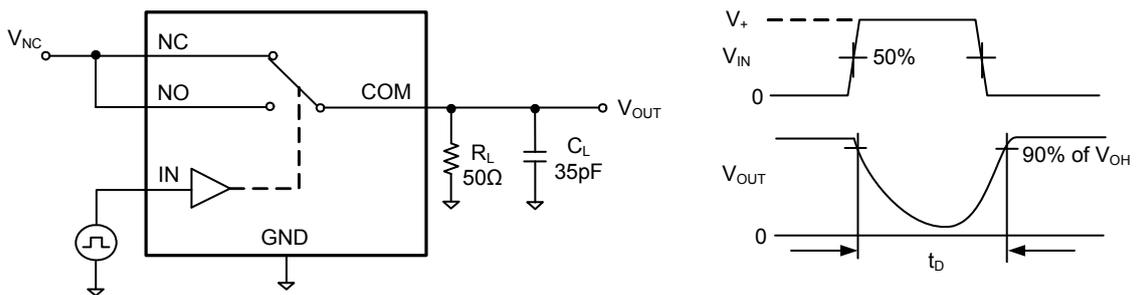
Test Circuit 3. Break-Before-Make Time Delay ( $t_D$ )
