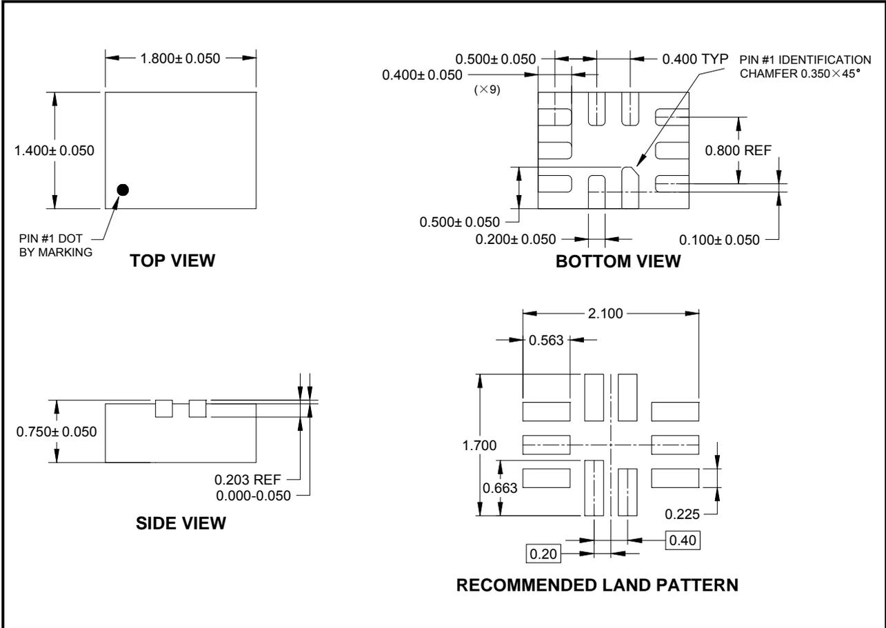
NOTE: All linear dimensions are in millimeters.
