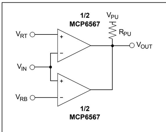
**FIGURE 4-13:** *Windowed Comparator.*
