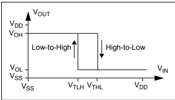
**FIGURE 4-7:** Hysteresis Diagram for the Inverting Circuit.
