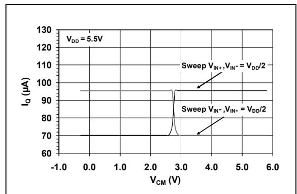
**FIGURE 2-18:** Quiescent Current vs. Common-mode Input Voltage.
