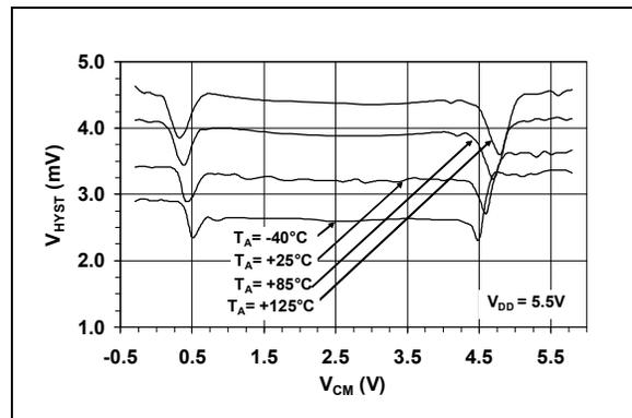
**FIGURE 2-12:** Input Hysteresis Voltage vs. Common-mode Input Voltage.
