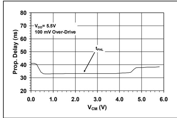
**FIGURE 2-34:** Propagation Delay vs. Common-mode Input Voltage.
