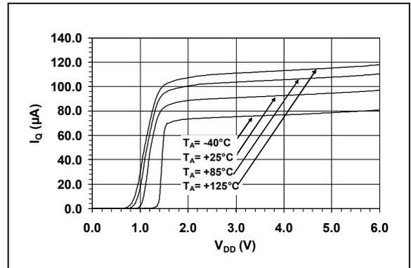
**FIGURE 2-17:** Quiescent Current vs. Supply Voltage vs. Temperature.
