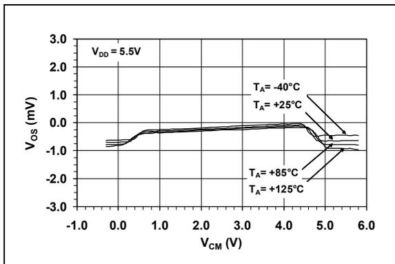
**FIGURE 2-9:** Input Offset Voltage vs. Common-mode Input Voltage.
