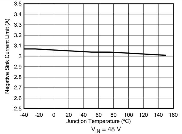
图 22. Sink Current Limit vs Temperature
