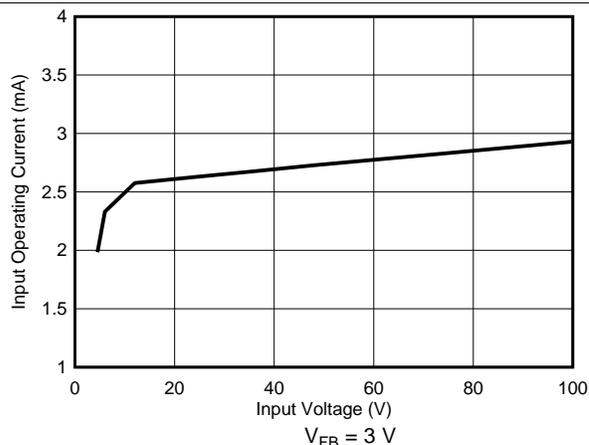
图 14.  $I_{IN}$  vs  $V_{IN}$  (Operating, Non Switching)
