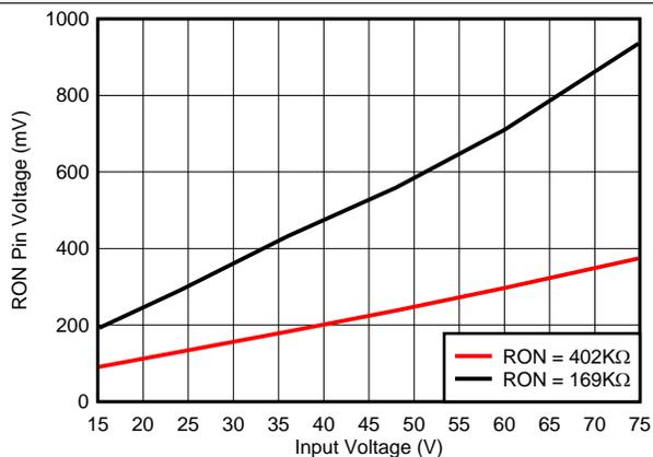
图 15. Voltage at RON pin vs Input Voltage
