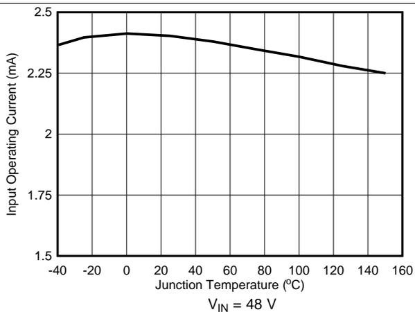
图 18. Input Operating Current vs Temperature
