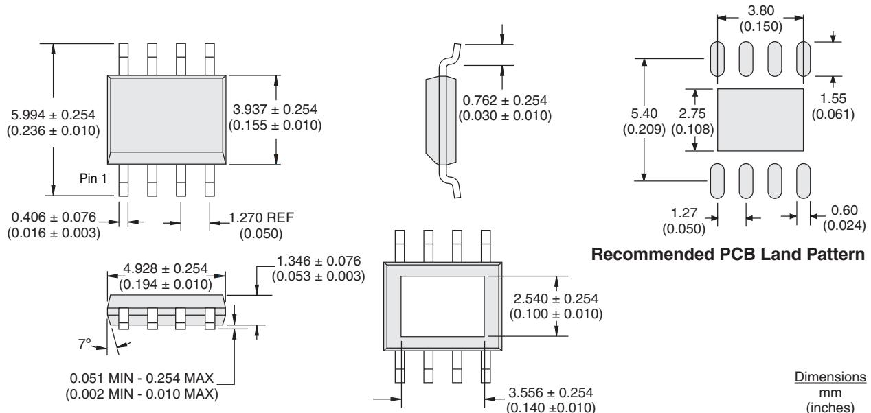
**Note:** The exposed metal pad on the back of the SI package should be connected to GND. It is not suitable for carrying current.
