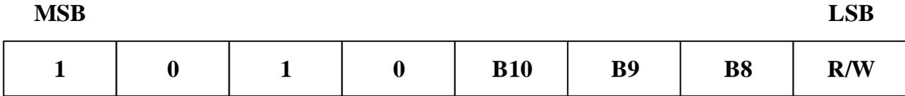
**Figure 5. Device Address**
