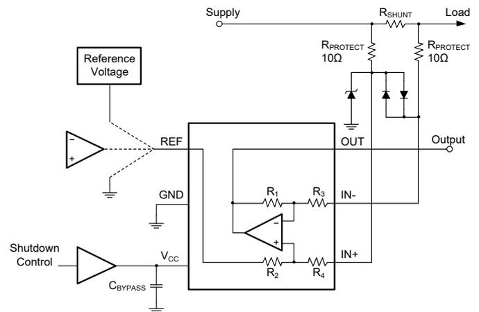
Figure 6. SGM8199 Transient Protection Using a Single Transzorb and Input Clamps
