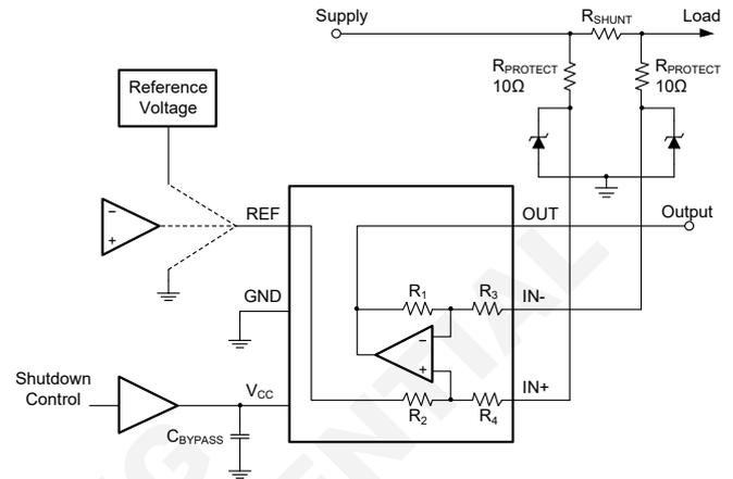
Figure 5. SGM8199 Transient Protection Using Dual Zener Diodes
